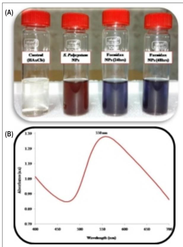
Fig. 3. Visual observation (A) and UV-visible spectra (B) of gold nanoparticles synthesized by fucoidan of *S. polycystum*
